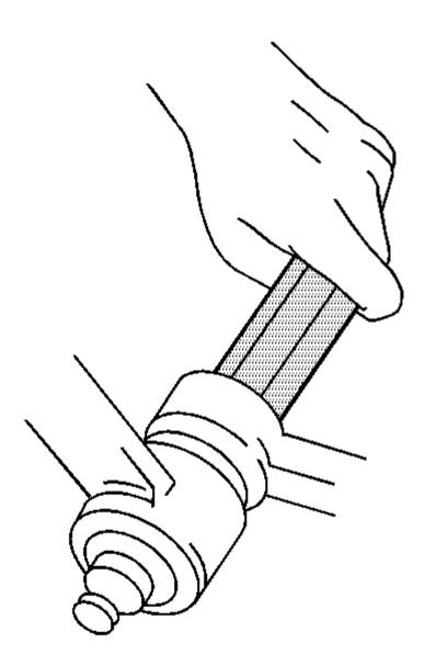
Fig. 26: Seating Relay Rod Tapers Courtesy of GENERAL MOTORS CORP.
