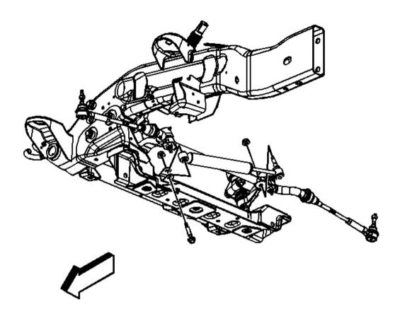
Fig. 19: Steering Damper Ball Stud Nut Courtesy of GENERAL MOTORS CORP.
