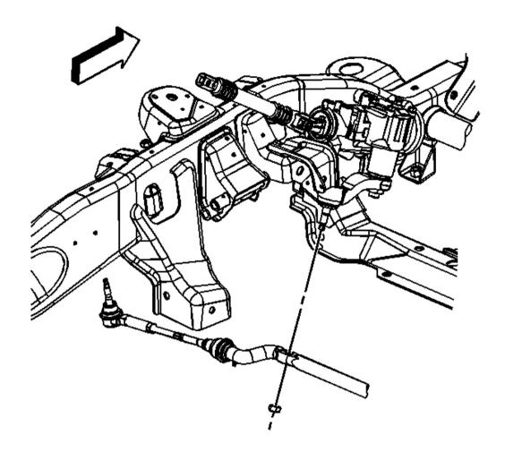
Fig. 12: Idler Arm Ball Stud Nut Courtesy of GENERAL MOTORS CORP.
