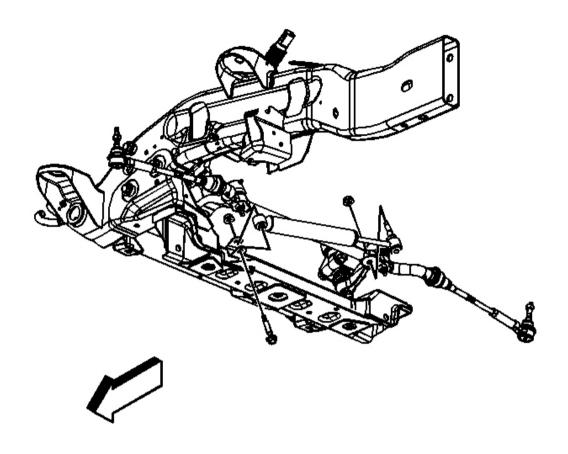
Fig. 20: Steering Damper Ball Stud Nut Courtesy of GENERAL MOTORS CORP.
