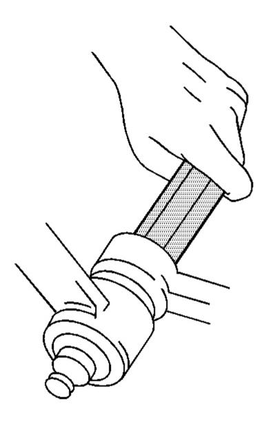
Fig. 5: Seating Relay Rod Tapers Courtesy of GENERAL MOTORS CORP.
