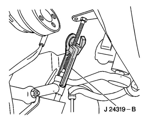
Fig. 23: Using J 24319-B To Remove Relay Rod From Pitman Arm Ball Stud Courtesy of GENERAL MOTORS CORP.
