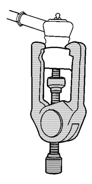
Fig. 2: Removing Outer Tie Rod Assembly From Steering Knuckle Courtesy of GENERAL MOTORS CORP.
