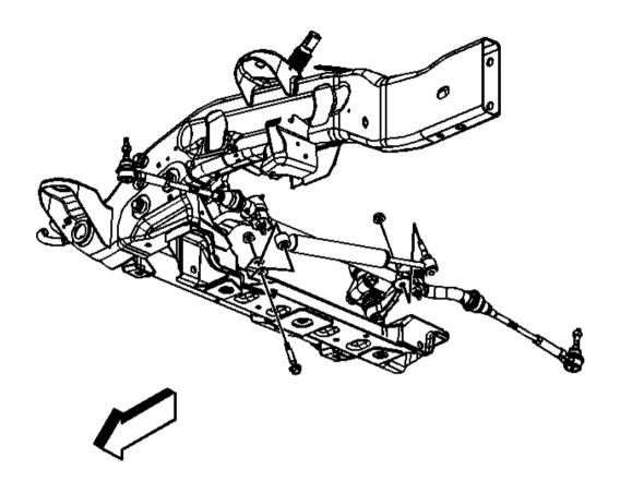
Fig. 17: Steering Damper Ball Stud Nut Courtesy of GENERAL MOTORS CORP.
