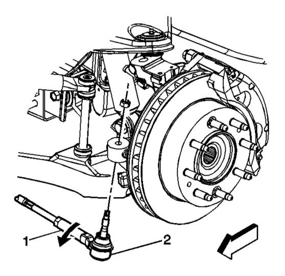
Fig. 1: Outer Tie Rod Ball Stud & Nut Courtesy of GENERAL MOTORS CORP.
