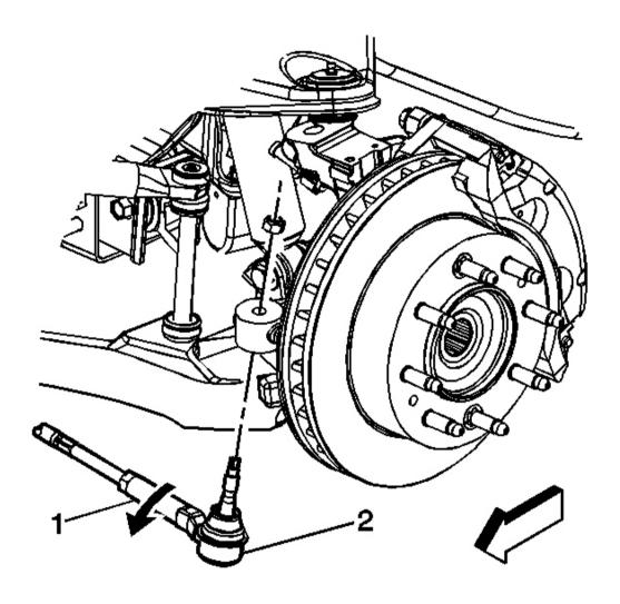
Fig. 3: Outer Tie Rod Ball Stud & Nut Courtesy of GENERAL MOTORS CORP.
