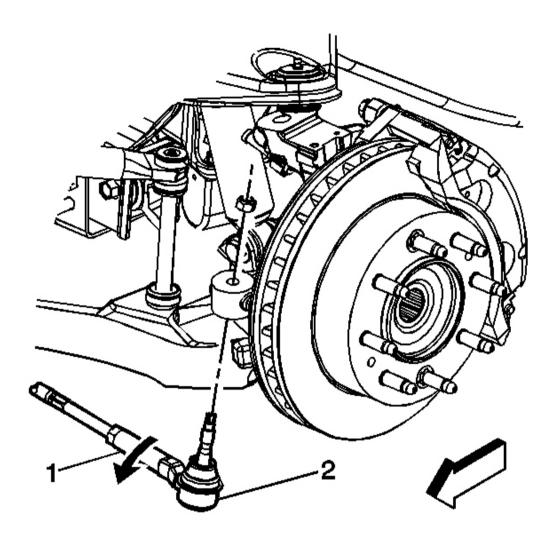
Fig. 4: Outer Tie Rod Ball Stud & Nut Courtesy of GENERAL MOTORS CORP.
