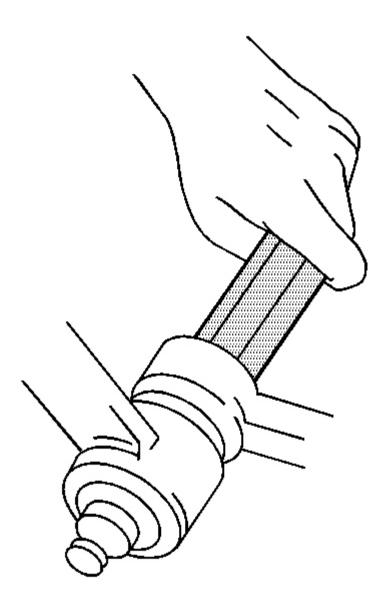
Fig. 21: Seating Relay Rod Tapers Courtesy of GENERAL MOTORS CORP.
