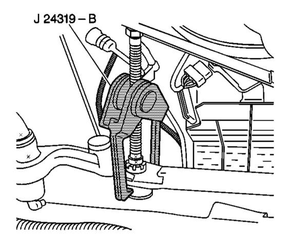
Fig. 18: Removing Steering Damper Ball Stud From Relay Rod Using J 24319-B Courtesy of GENERAL MOTORS CORP.
