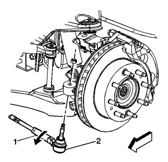
Fig. 6: Outer Tie Rod Ball Stud & Nut Courtesy of GENERAL MOTORS CORP.
