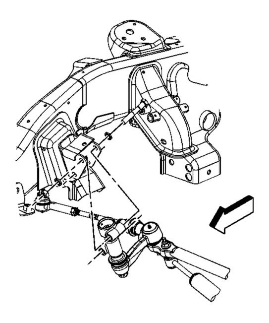
Fig. 10: View Of Idler Arm Courtesy of GENERAL MOTORS CORP.
