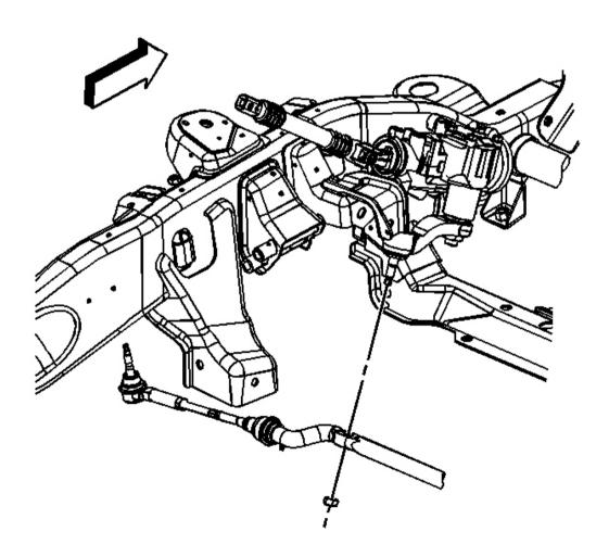
Fig. 25: Idler Arm Ball Stud Nut Courtesy of GENERAL MOTORS CORP.
