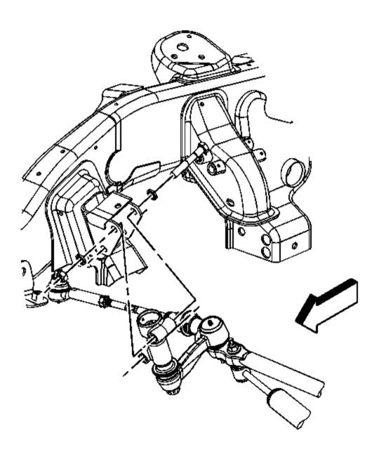
Fig. 15: View Of Idler Arm Courtesy of GENERAL MOTORS CORP.
