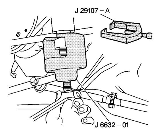
Fig. 24: Using J 29107-A Or J 6632-01 To Remove Pitman Arm From Steering Gear Pitman Shaft Courtesy of GENERAL MOTORS CORP.
