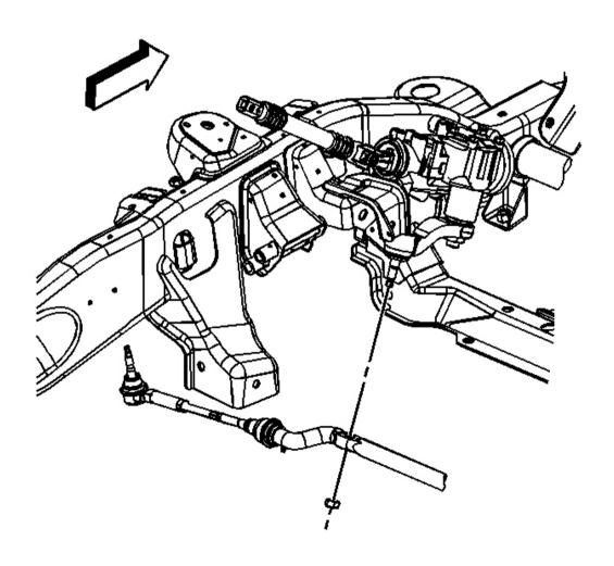
Fig. 14: Idler Arm Ball Stud Nut Courtesy of GENERAL MOTORS CORP.
