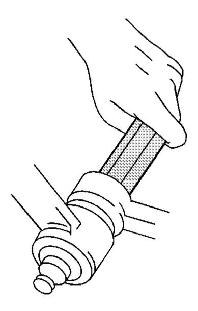
Fig. 16: Seating Relay Rod Tapers Courtesy of GENERAL MOTORS CORP.
