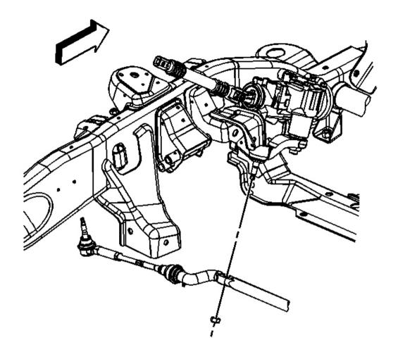
Fig. 22: Idler Arm Ball Stud Nut Courtesy of GENERAL MOTORS CORP.
